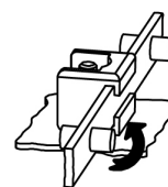
3. By tightening the nut the living hinge automatically and securely attaches the flat rod..
